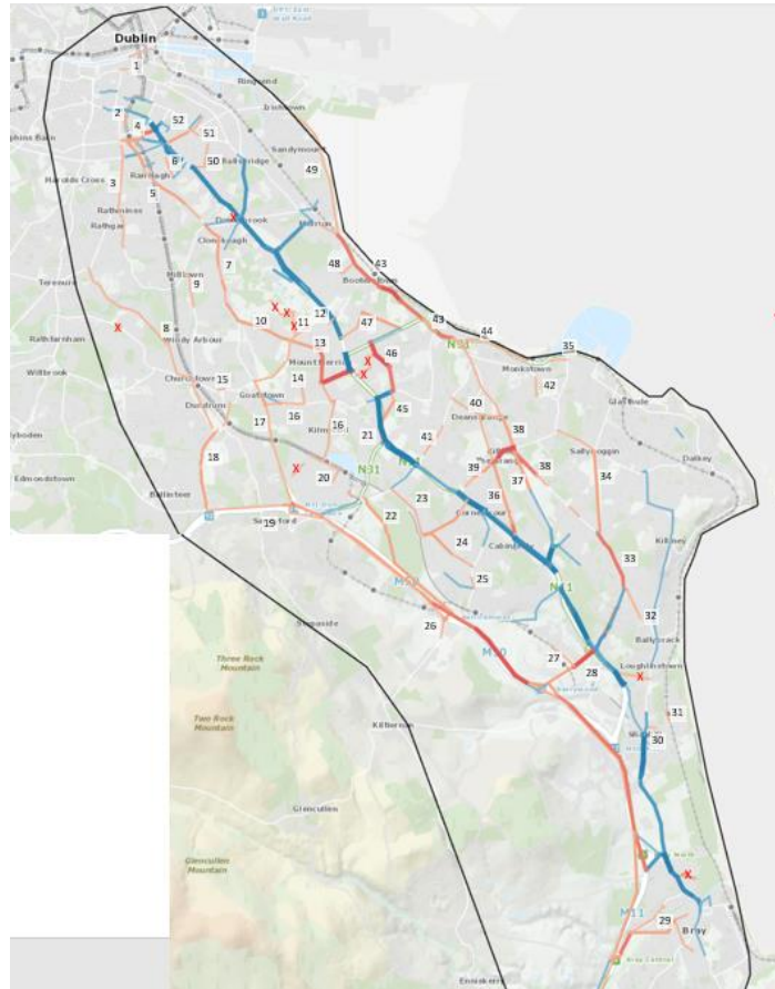
Figure 5.8: Flow Difference on Road links (Do Minimum vs Do Something), PM Peak Hour, 2028 Opening Year
