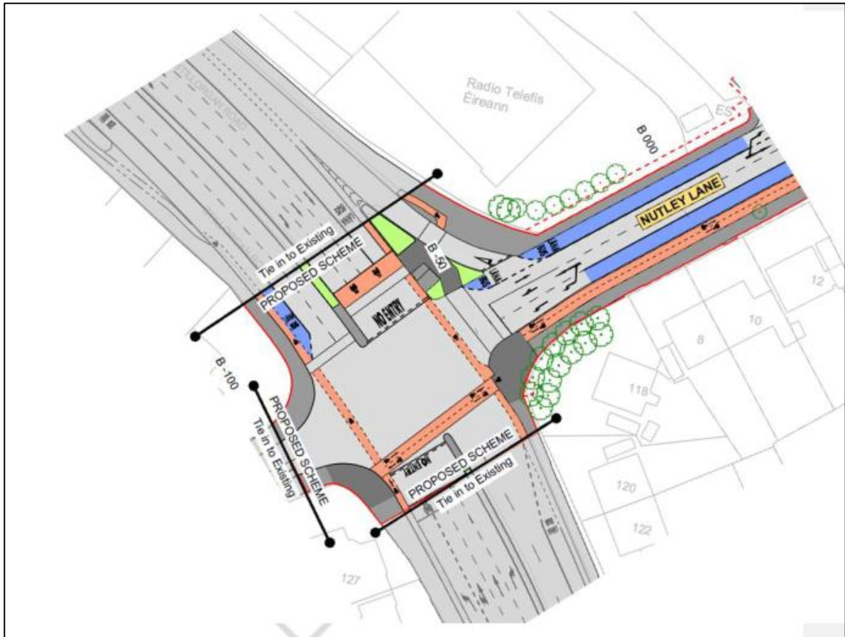
Figure 3.26 Preliminary Design of the Belfield/ Blackrock to City Centre CBC Scheme at Nutley Lane, tying into the existing R138 Stillorgan Rd/Nutley Lane junction layout
