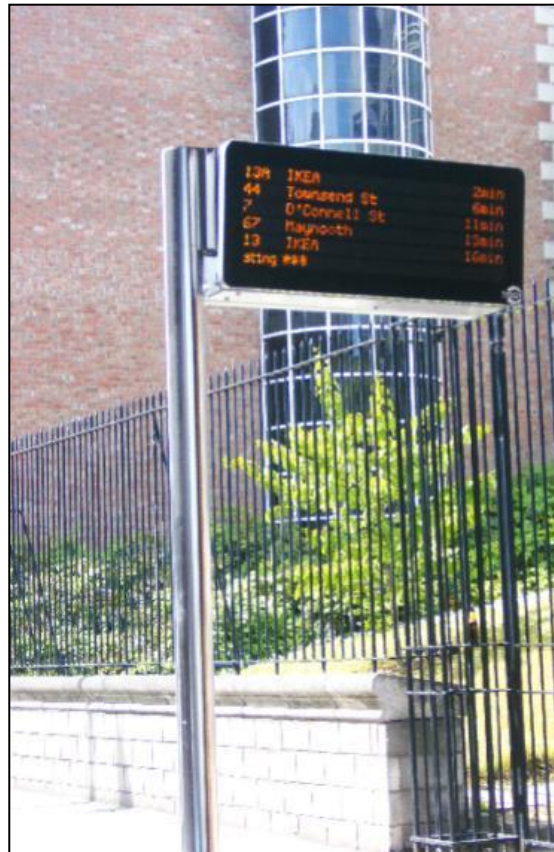
Figure 12.1: RTPI Display at Bus Stop
